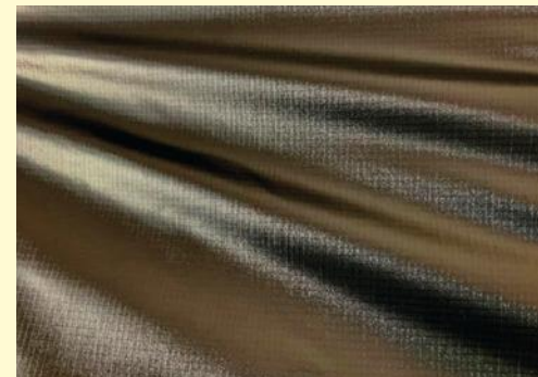
20d mini-ripstop nylon fabric with a titanium spattering finish from Craftevo
